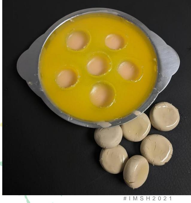
5. On a sheet tray or other flat surface, stretch power mesh and pour red rubber on top to cover the sheet. The Power Mesh adds durability to the bottom to prevent bubbling when filling later. While the rubber is wet, add as many pads as possible to minimize waste. Allow to cure.
