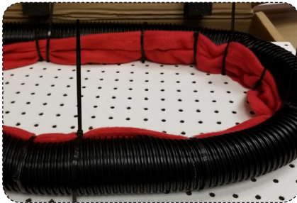
Figure 5.41 – Vacuum hose tied around and down onto the plywood sheet using zip ties
