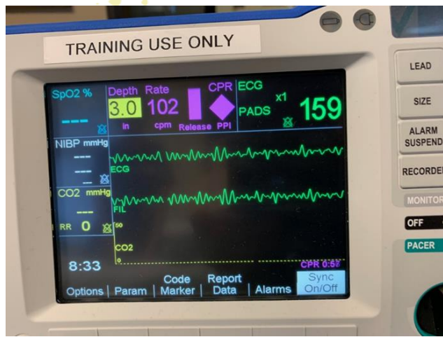
External accelerometer measurement Real CPR Help, ZOLL® R series® defibrillator
