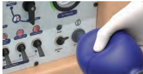
Air reservoir is charged using the supplied manual pump or a BVM
