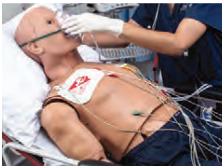
Attach real electrodes and view HAL's ECG generated in real-time. HAL's ECG features physiologic variations in rhythm, never repeating textbook patterns
